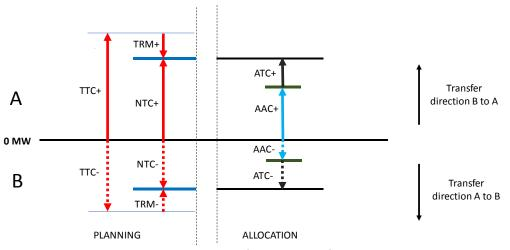
Figure SDC 1. Transfer capacity definitions
