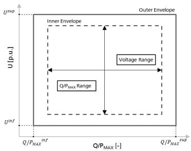
Figure CC 14. U-Q/P<sub>MAX</sub>-profiles to be defined by the relevant **TSO**.
