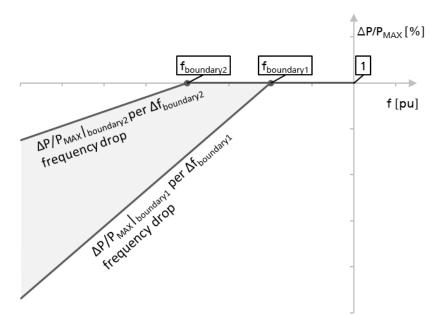
*Figure CC 2. Maximum power capability reduction with falling frequency. The percentage value of the reduction refers to the maximum active power of Synchronous Power-Generating Module.*
