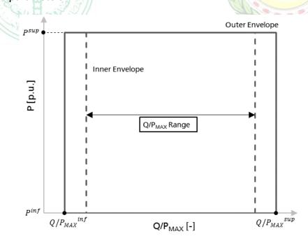
Figure CC 8. P-Q/P<sub>MAX</sub>-profile to be defined by the relevant **TSO** for Inverter-based Power-Generating Modules.
