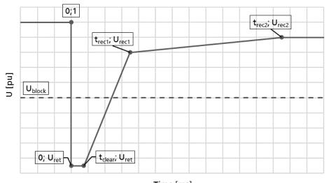
Time [ms] Figure CC 9. Fault-ride-through profile of an HVDC Converter Station.
