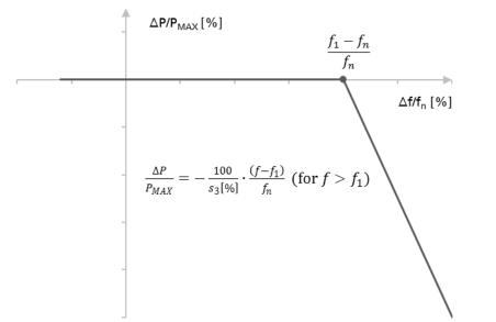
Figure CC 12. Active power frequency response capability of HVDC System in LFSM-O mode.
