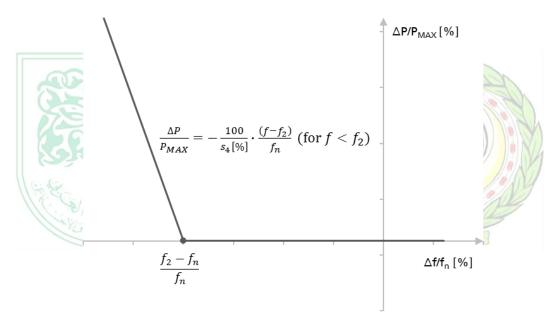
Figure CC 13. Active power frequency response capability of HVDC System in LFSM-U mode.
